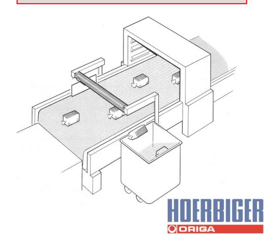
Origa Rodless Cylinders Work: Bakery Ejector
